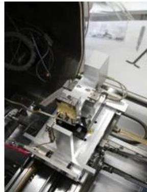
Compression of lattice structures inside the SEM
