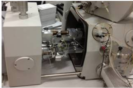
Tension, compression or bending inside the SEM with HR-DIC strain field measurements
